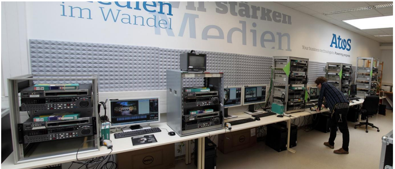
The ATOS Installation at ORF using NOA Framelector multichannel video ingest systems
